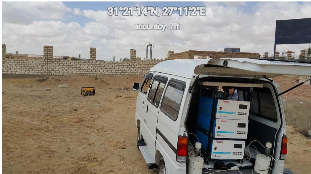
Figure 3-1 ambient air quality monitoring system
