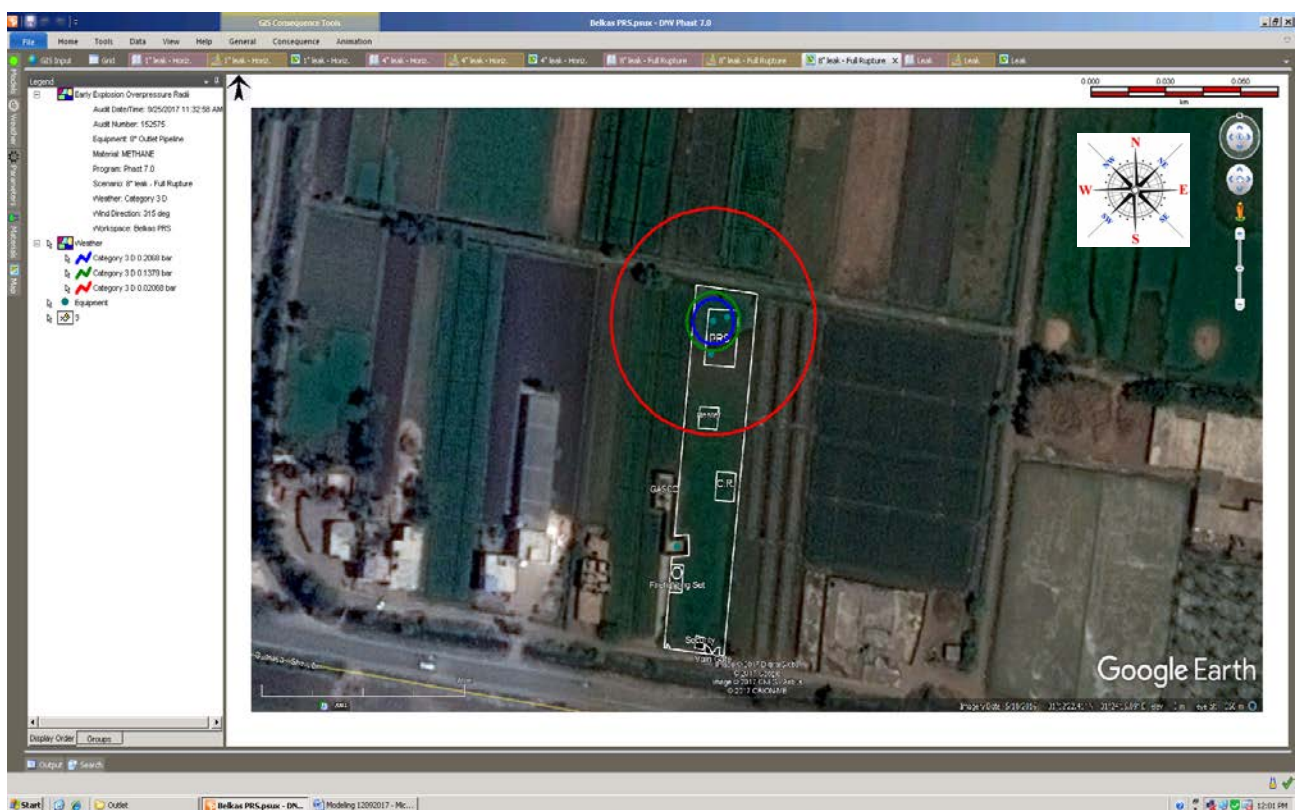
Figure (37) Early Explosion Overpressure Waves (8" Outlet Pipeline Full Rupture)
