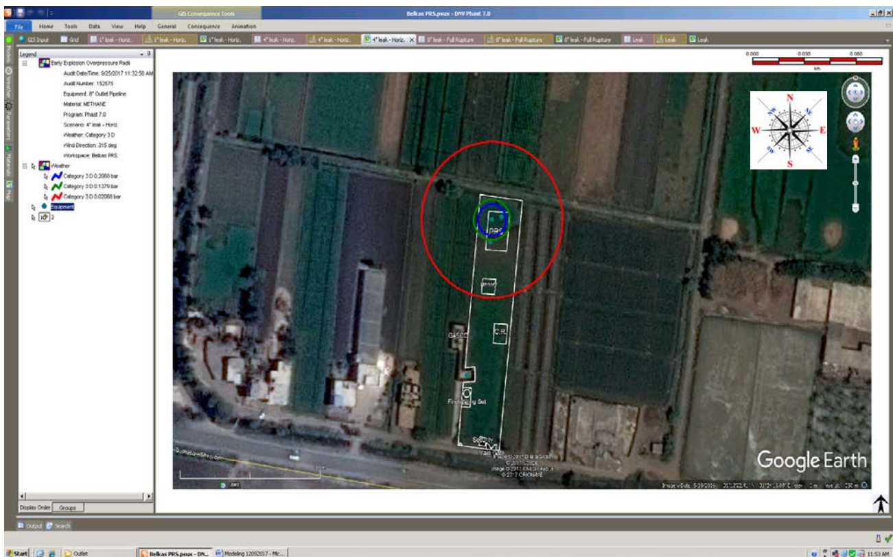
Figure (33) Early Explosion Overpressure Waves (4" hole in 8" Outlet Pipeline)
