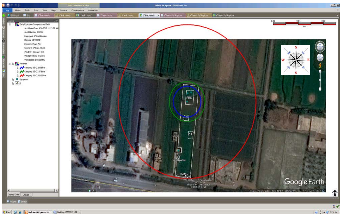
Figure (21) Early Explosion Overpressure Waves (3" hole in 6" Inlet Pipeline)
