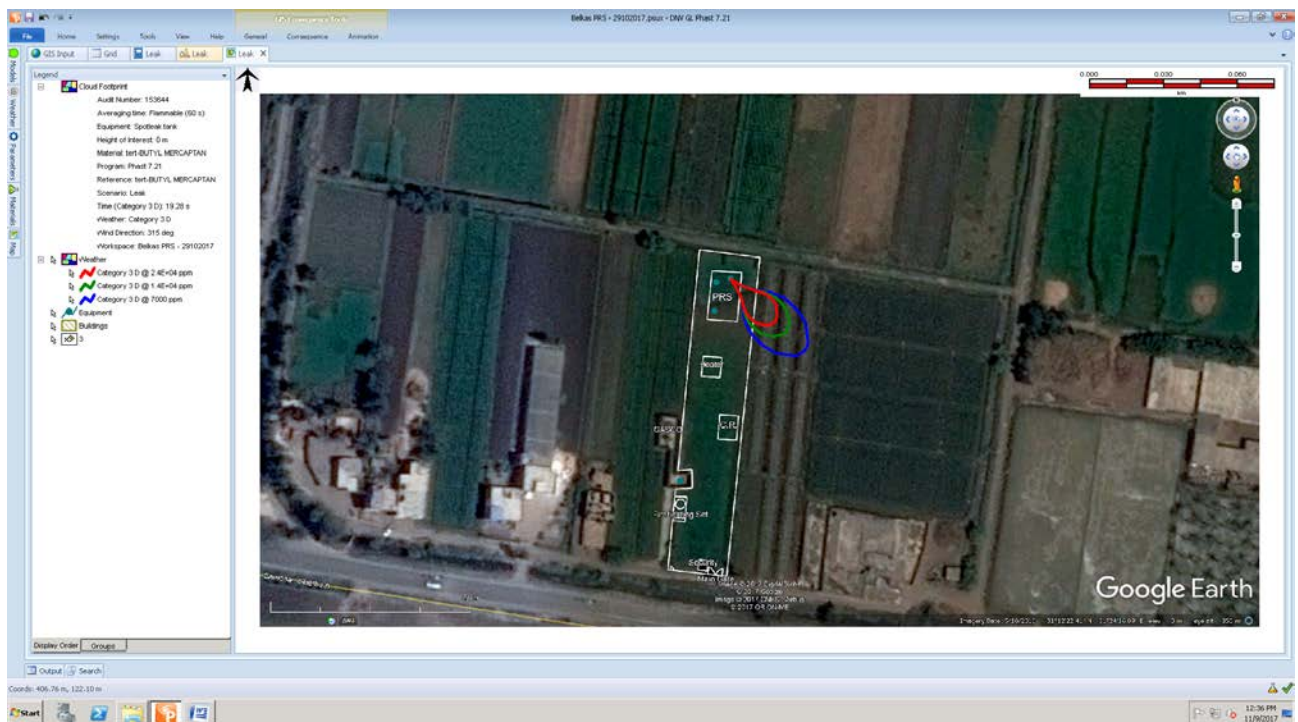
Figure (41) Vapor Cloud (UFL/LFL) Footprint on Site (Odorant leak)
