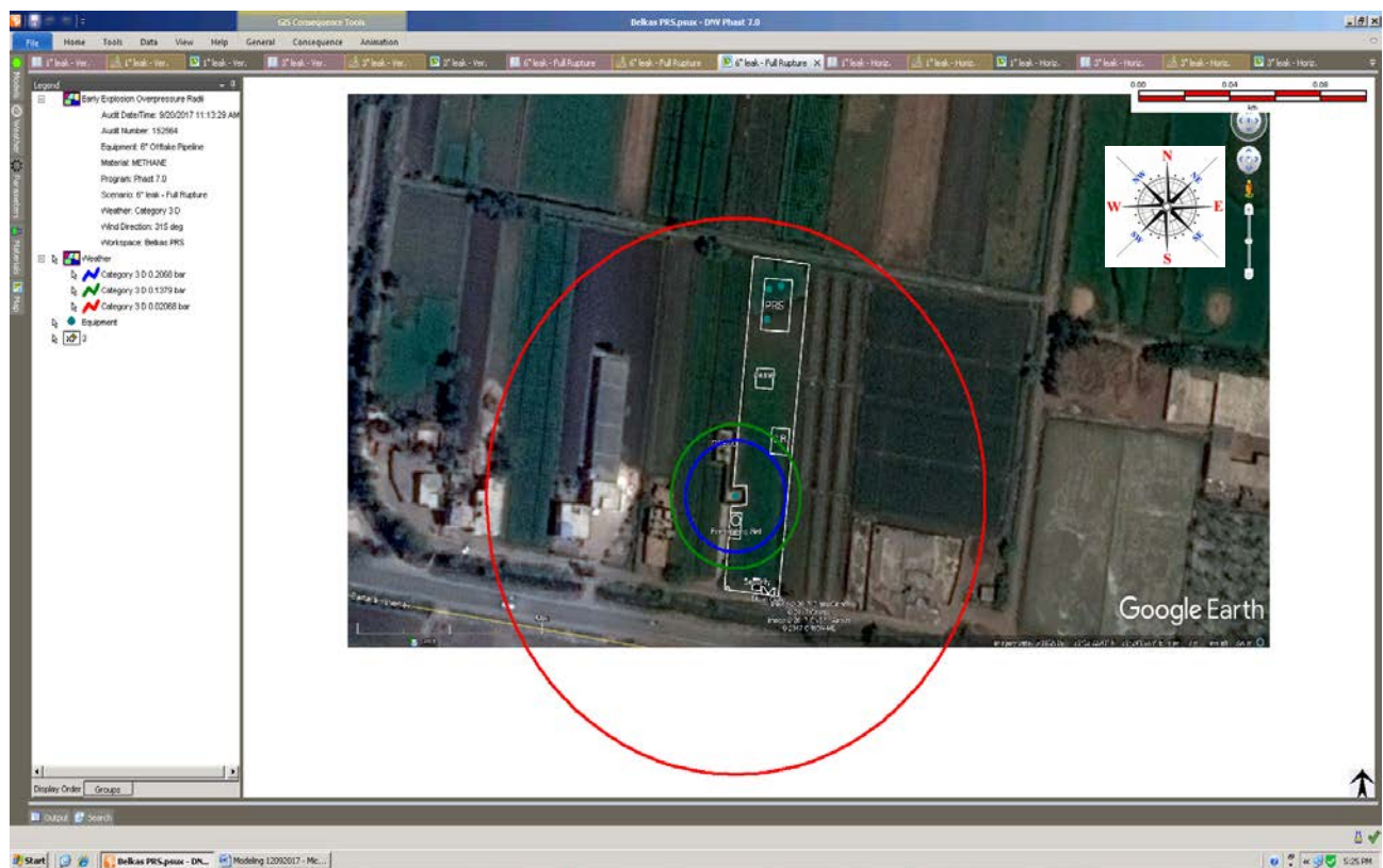
Figure (53) Early Explosion Overpressure Waves (6" off-take Pipeline Full Rupture)
