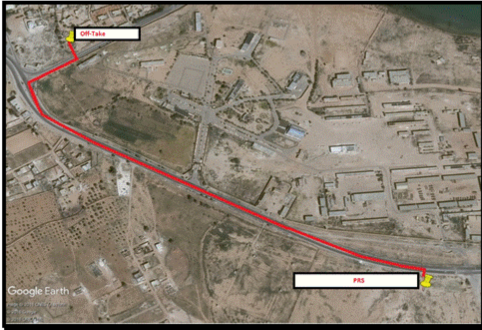
Figure 2-5: Existing Matrouh inlet connection / pipeline “70bar system”
