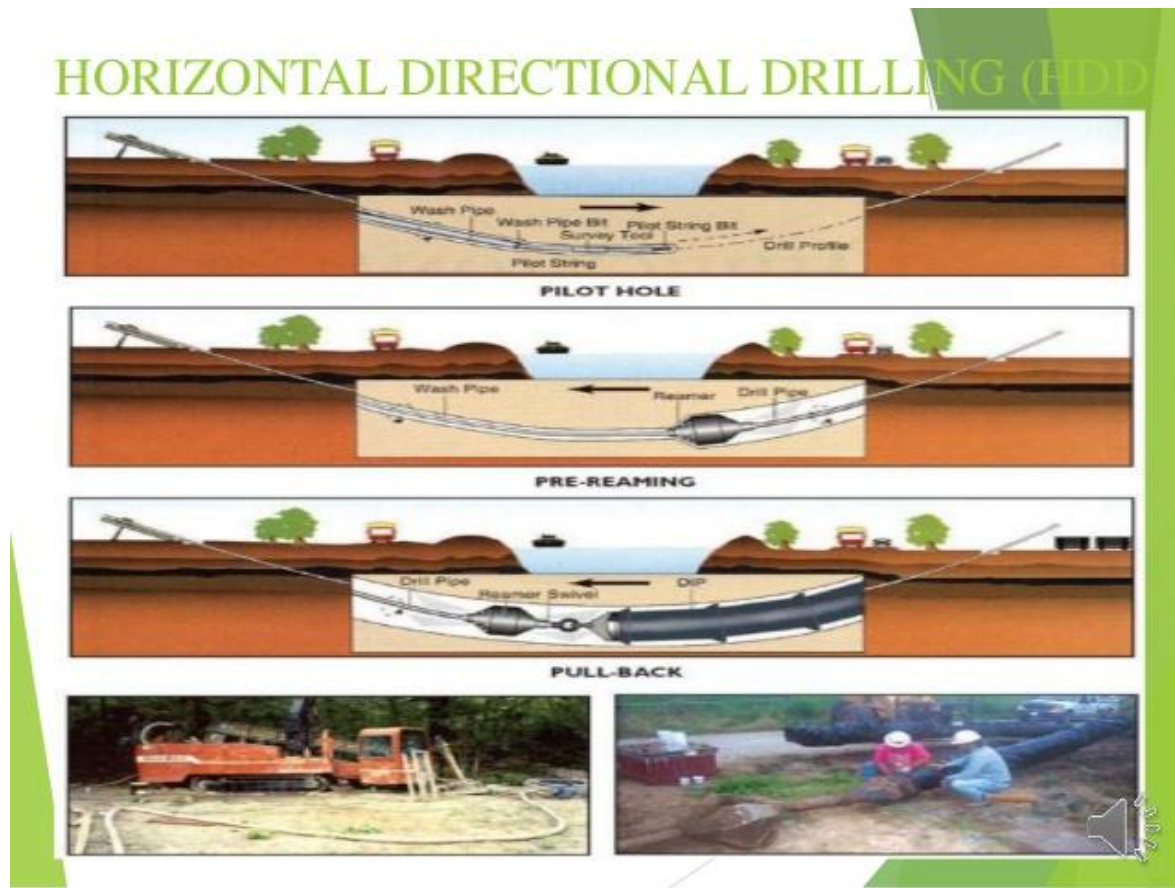
Figure 5-3: Horizontal Directional Drilling
