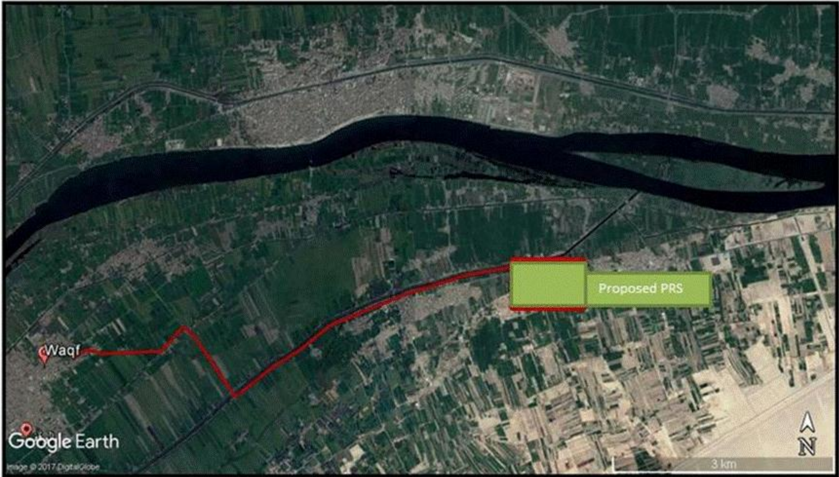
Figure 2-3: Intermediate Pressure Network - Main feeding line/network “4- 7 bar system Connecting the new PRS to the city regulator in Waqf
