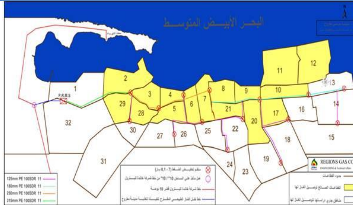
Figure 2-2 The 7 Bar network- ( network sectors)
