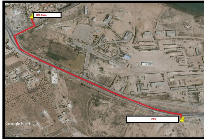
Figure 2-5: Existing Matrouh inlet connection /pipeline”70bar system”
