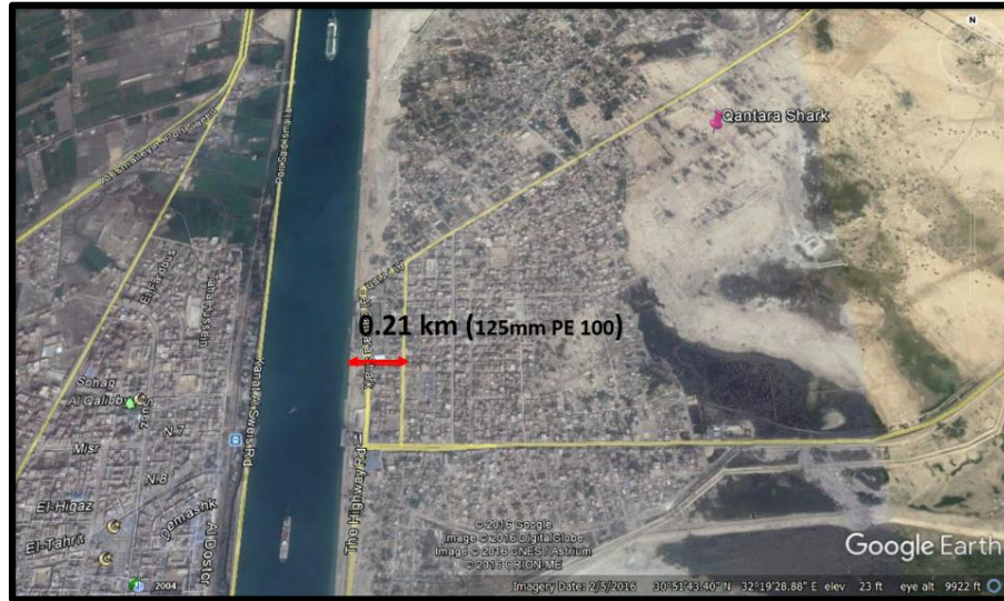
Figure 4-8 The closest intermediate pressure line (125mm PE 100) to the Suez Canal at a distance of 210 m
