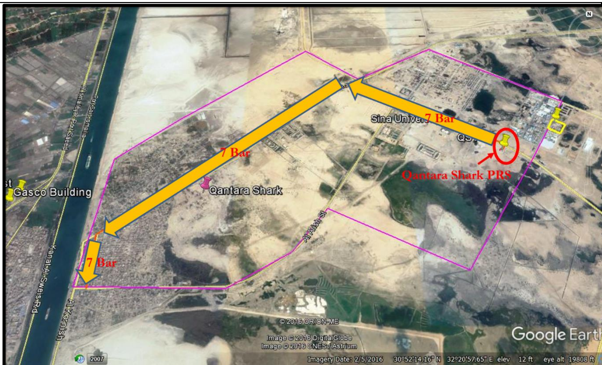
Figure 2-3 Intermediate Pressure Network's routing within the borders of QS Source: Study team
