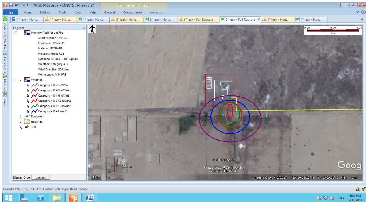
Figure (18) Heat Radiation Contours from Jet Fire (6" Inlet Pipeline Full Rupture)
