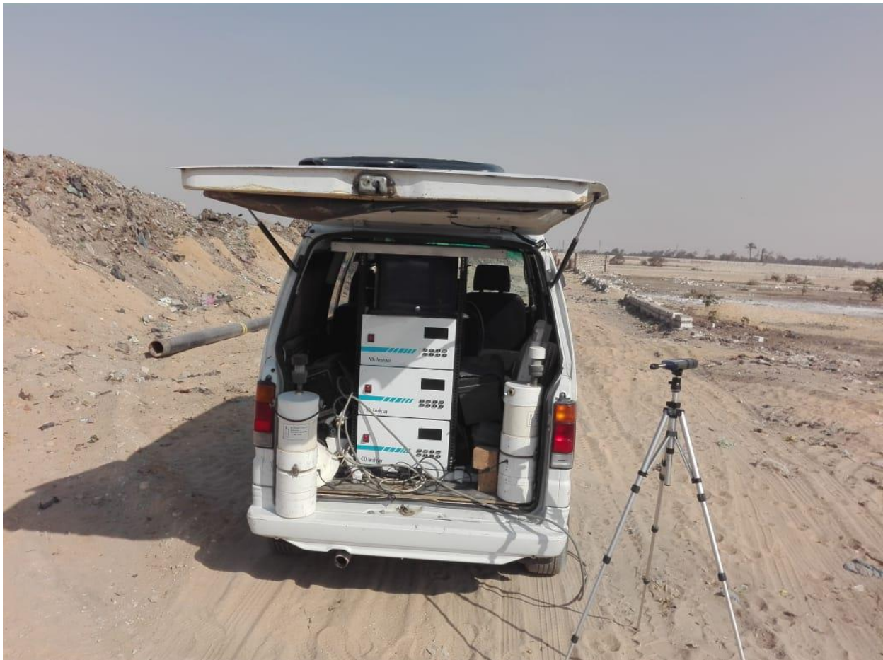
Figure 3-1 ambient air quality monitoring system
