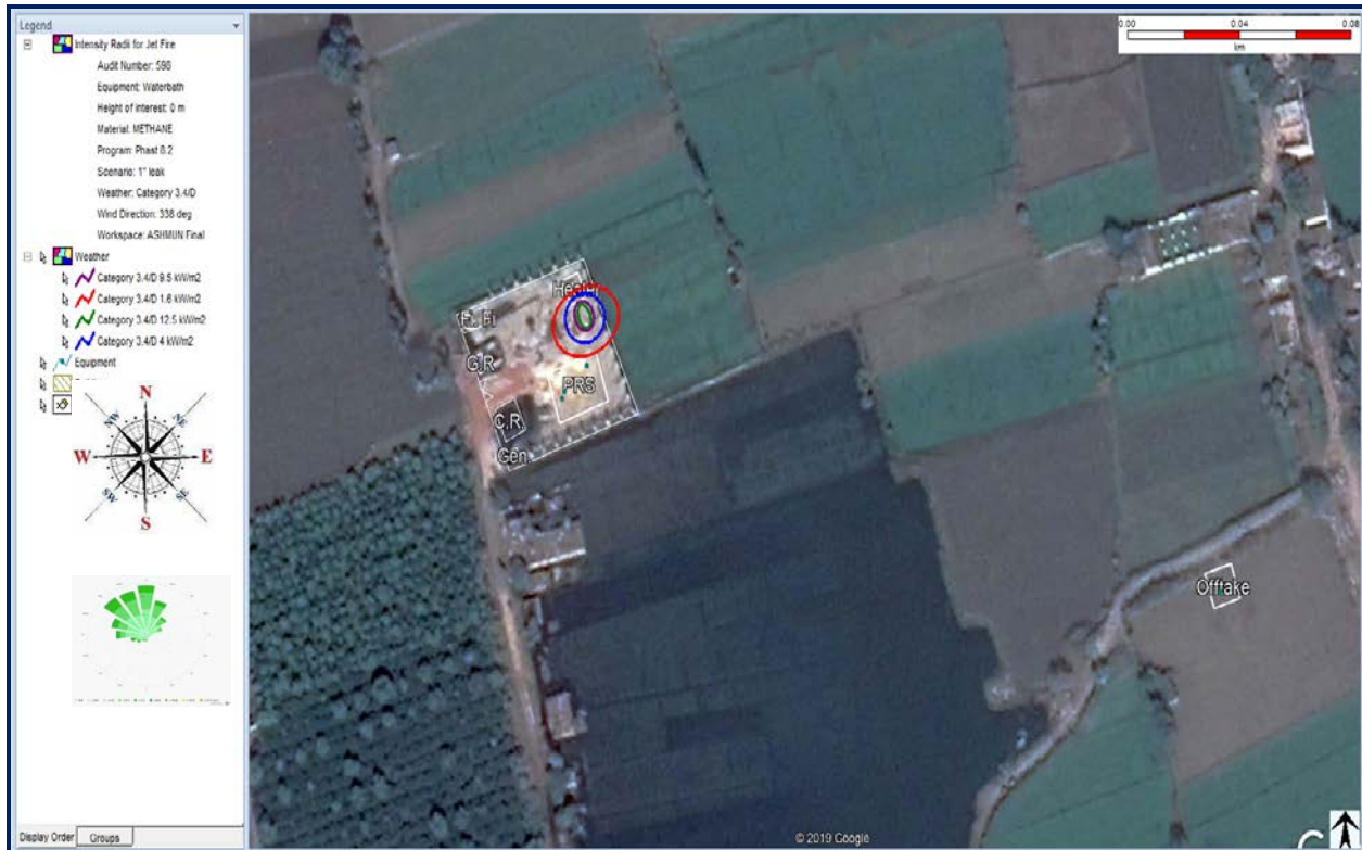
Figure (39) Heat Radiation Contours - Fire on Site (Gas Heater)
