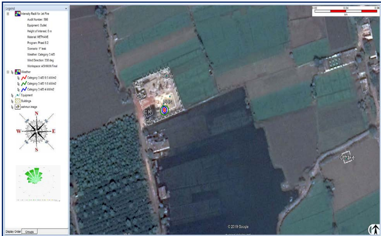
Figure (23) Heat Radiation Contours from Jet Fire (1" hole in 6" Outlet Pipeline)
