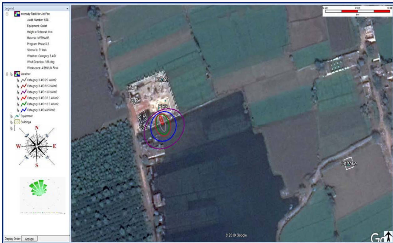
Figure (25) Heat Radiation Contours from Jet Fire (3" hole in 6" Outlet Pipeline)
