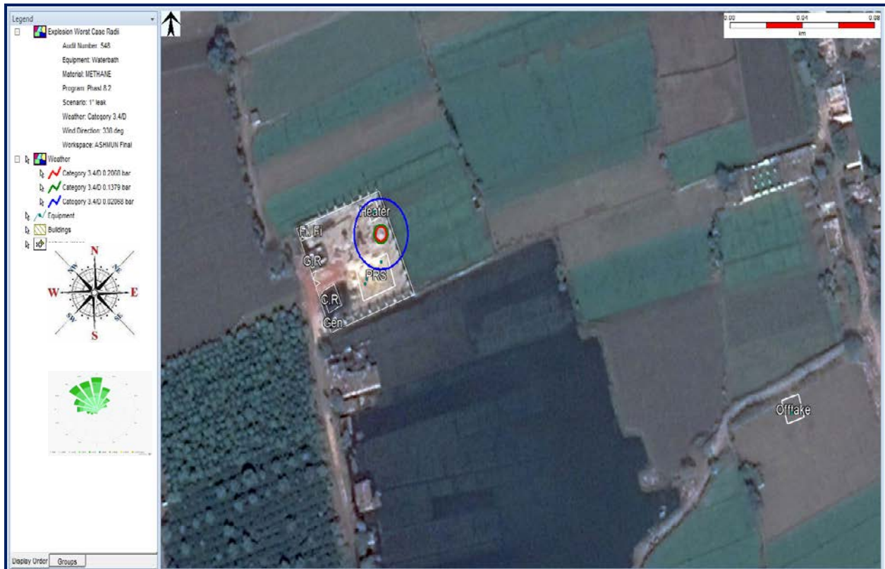
Figure (41) Late Explosion Overpressure Waves on Site (Gas Heater)
