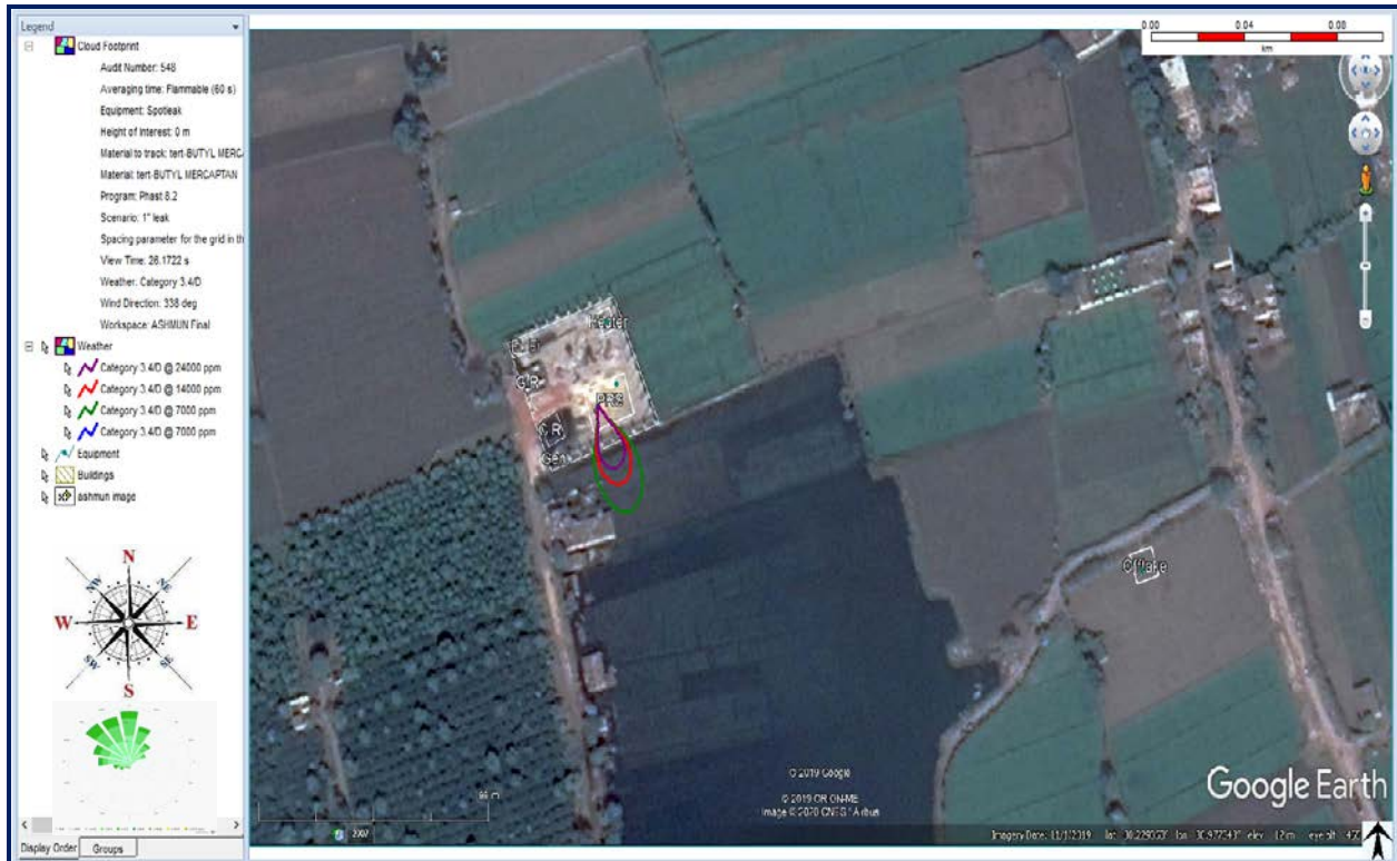
Figure (32) Cloud Footprint (UFL/LFL) on site (Odorant leak)
