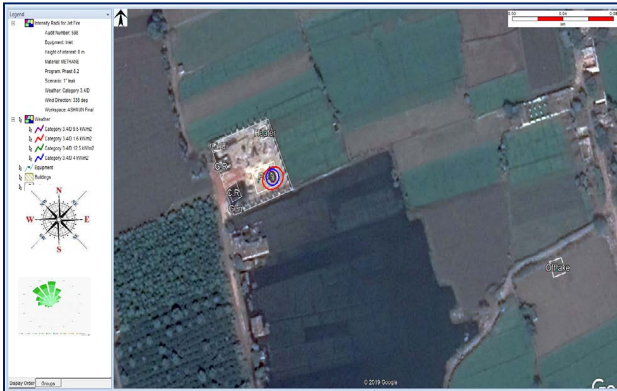
Figure (15) Heat Radiation Contours from Jet Fire (1" hole in 4" Inlet Pipeline)
