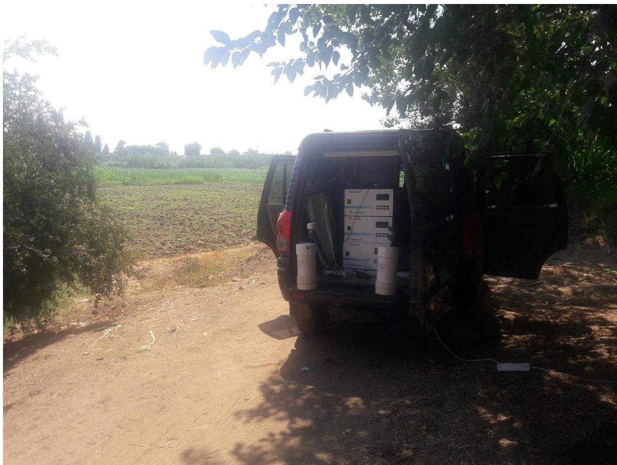
Figure 3-1 ambient air quality monitoring system
