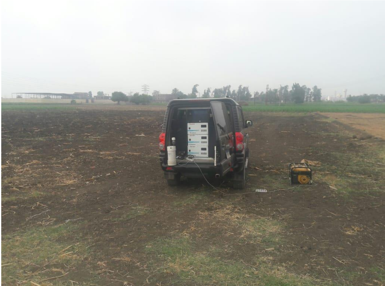
Figure 3-1 ambient air quality monitoring system
