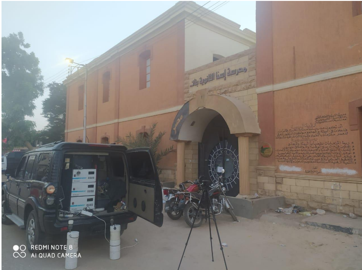
Figure 3-1 ambient air quality monitoring system
