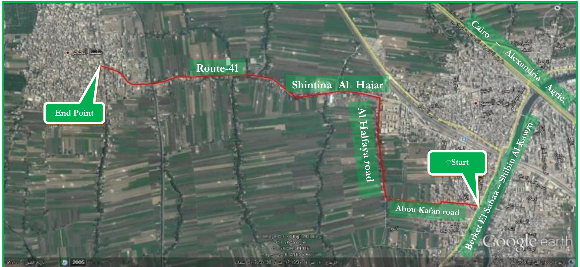
Figure 2-3: Satellite Map showing the proposed pipeline route feeding Shintina Al Hajar & Um Saleh areas
