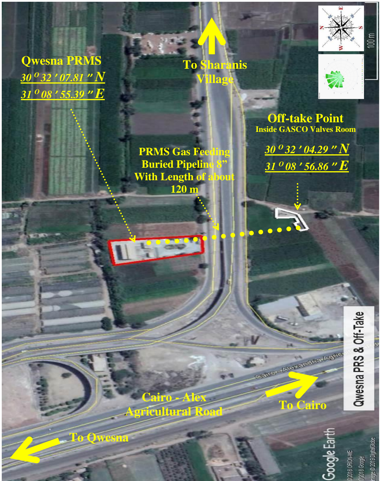
Figure (8) Qwesna PRMS, Gas Feeding Pipeline and Off-Take Point Plot Plan Plotted on Google Earth Photo
