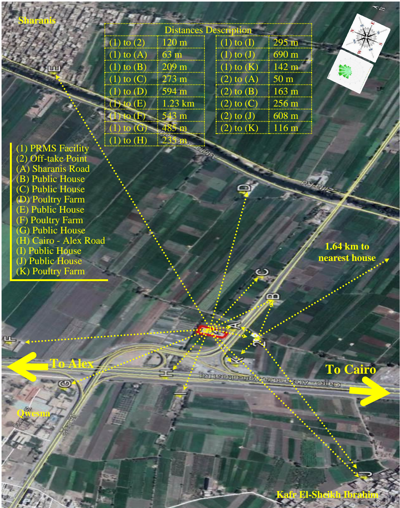
Figure (12) Qwesna Pressure Reduction Station and Off-take Point Show Surroundings Plotted on Google Earth Photo
