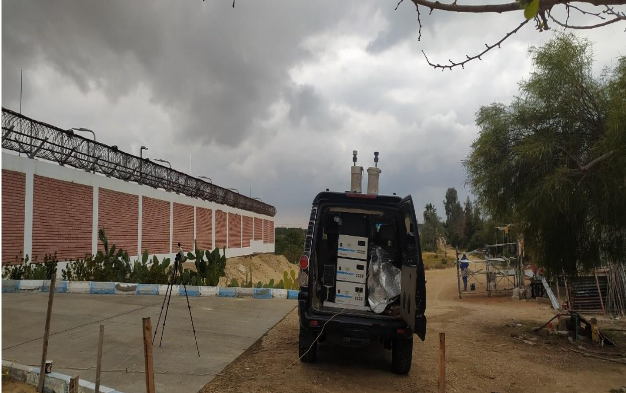
Figure 3-1 ambient air quality monitoring system
