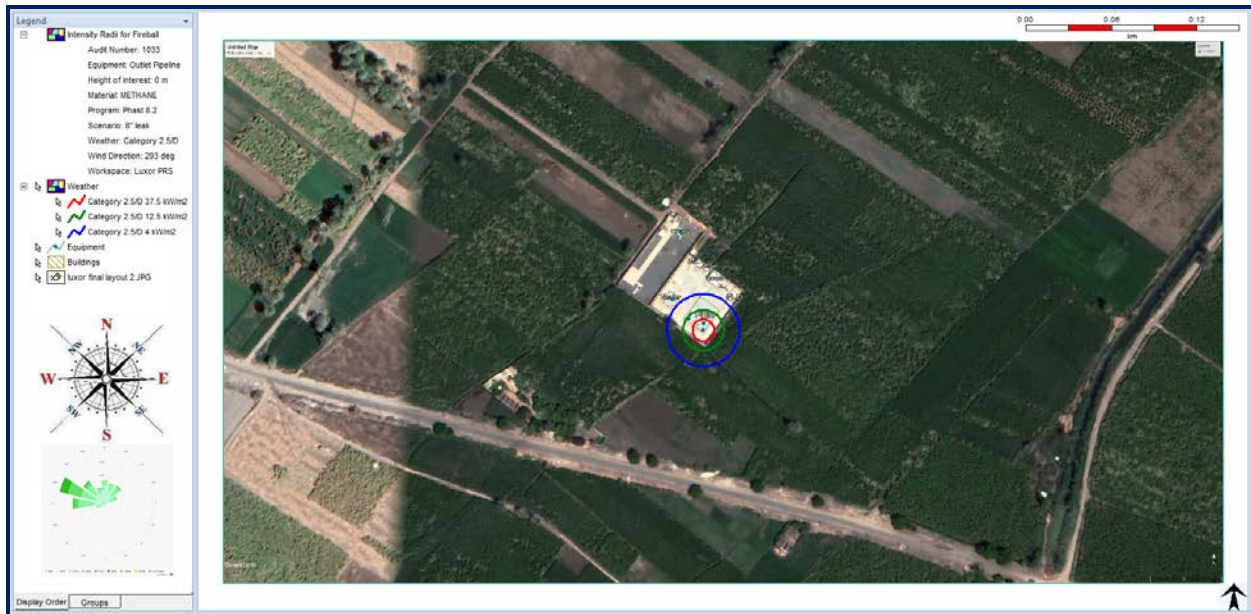
Figure 28. Heat Radiation Contours from Fireball (8'' Outlet Pipeline Full Rupture)
