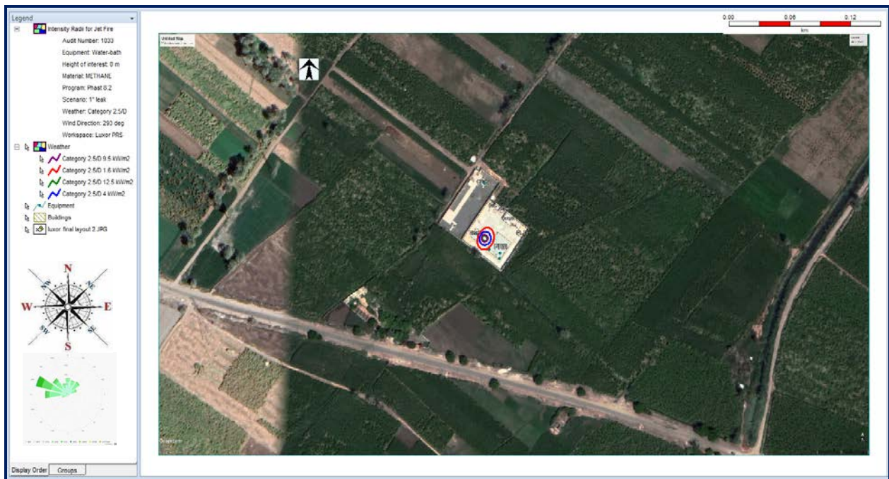
Figure 37. Heat Radiation Contours - jet Fire on Site (Gas Heater)
