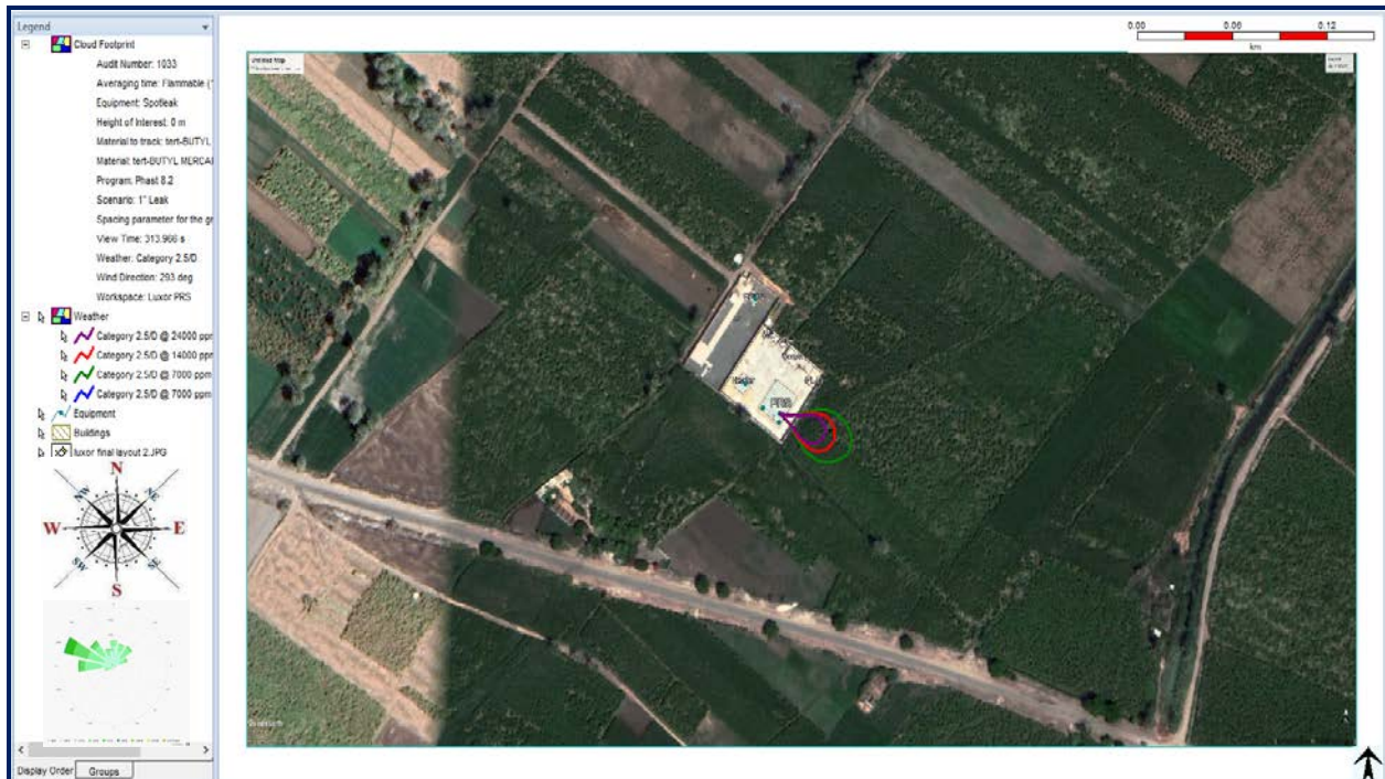
Figure 30. Cloud Footprint (UFL/LFL) on site (Odorant leak)
