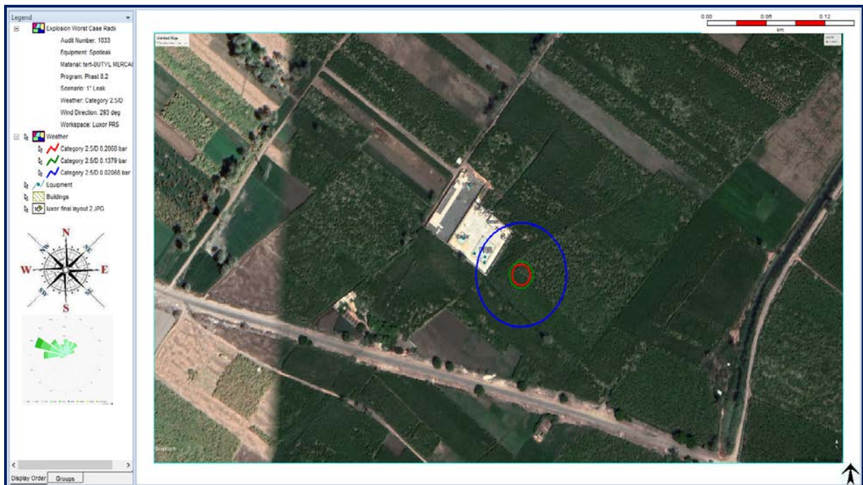
Figure 34. Worst-case Explosion Overpressure Waves on Site (Odorant Leak)
