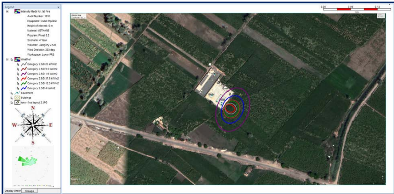
Figure 23. Heat Radiation Contours from Jet Fire (4'' hole in 8'' Outlet Pipeline)
