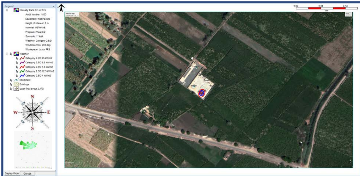
Figure 12. Heat Radiation Contours from Jet Fire (1" hole in 8" Inlet Pipeline)
