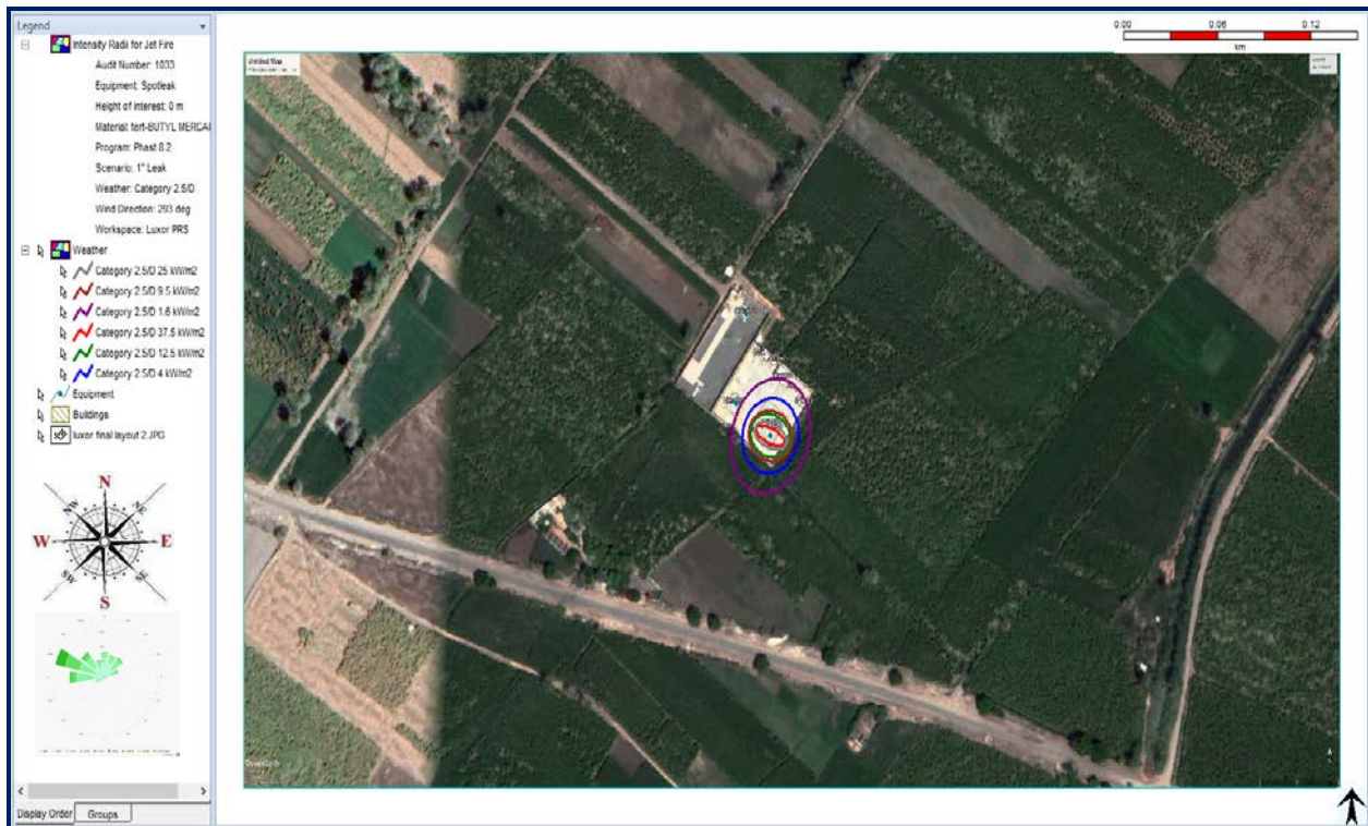
Figure 32. Heat Radiation Contours - Jet Fire on Site (Odorant Leak)
