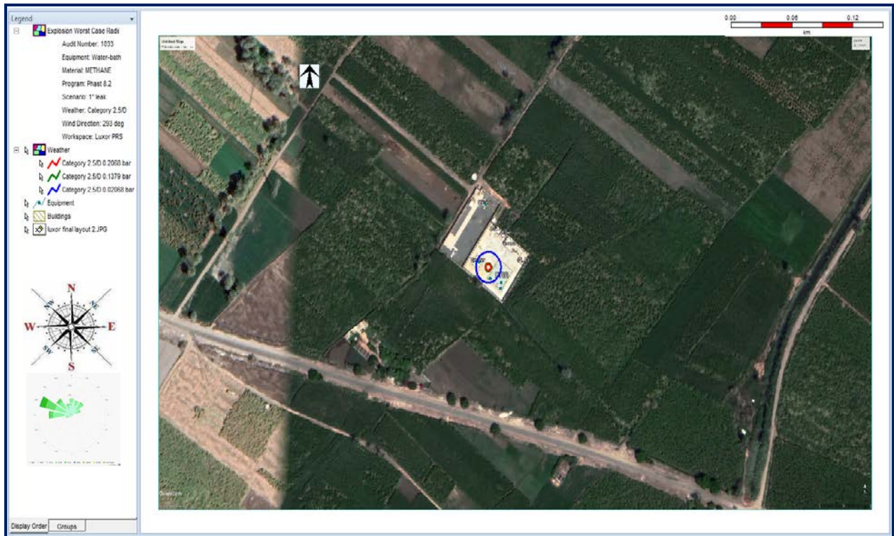
Figure 39. Worst-case Explosion Overpressure Waves on Site (Gas Heater)
