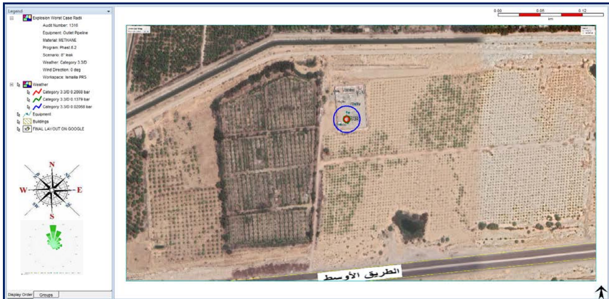
Figure 26. Worst-Case Explosion Overpressure Waves (8'' Outlet Pipeline Full Rupture)
