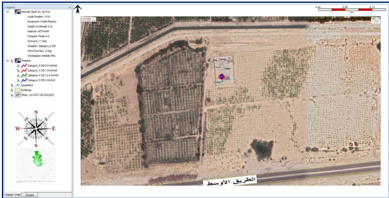
Figure 20. Heat Radiation Contours from Jet Fire (1" hole in 8" Outlet Pipeline)
