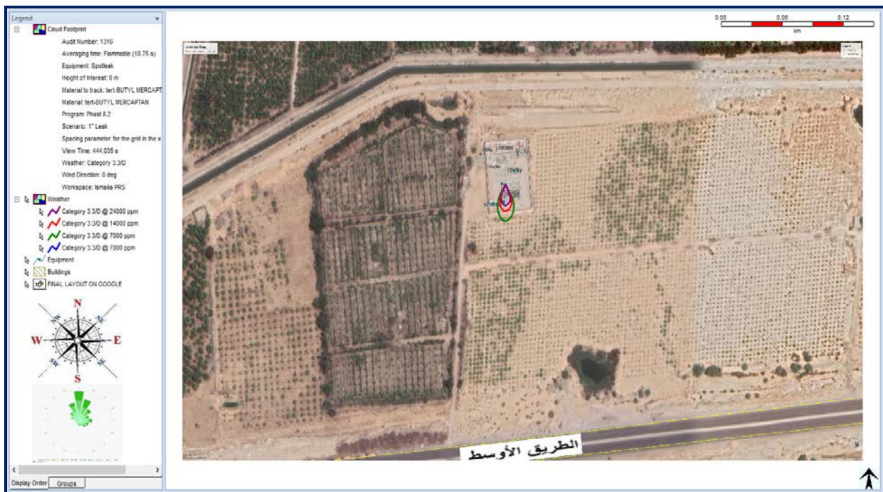
Figure 29. Cloud Footprint (UFL/LFL) on site (Odorant leak)
