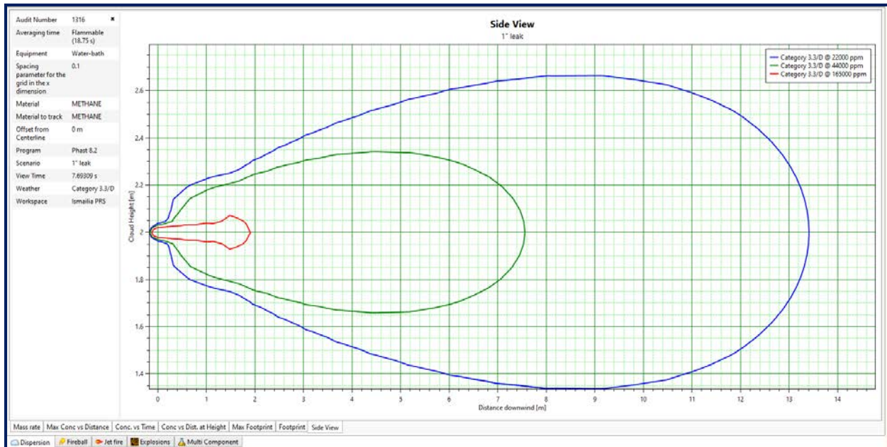
Figure 34. Vapor Cloud (UFL/LFL) Side View Graph (Gas Heater)
