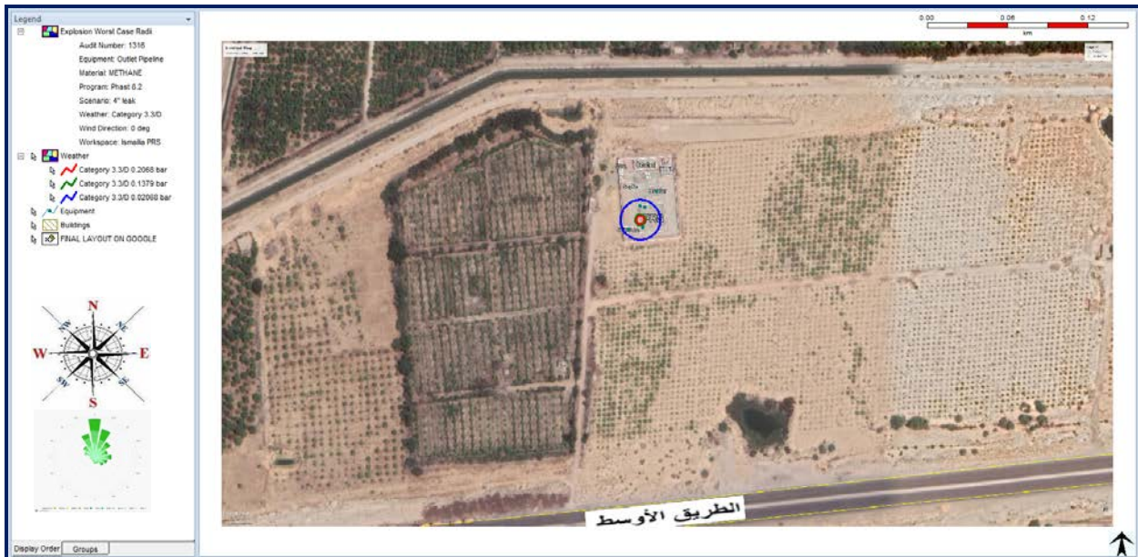
Figure 23. Worst-Case Explosion Overpressure Waves (4'' hole in 8'' Outlet Pipeline)
