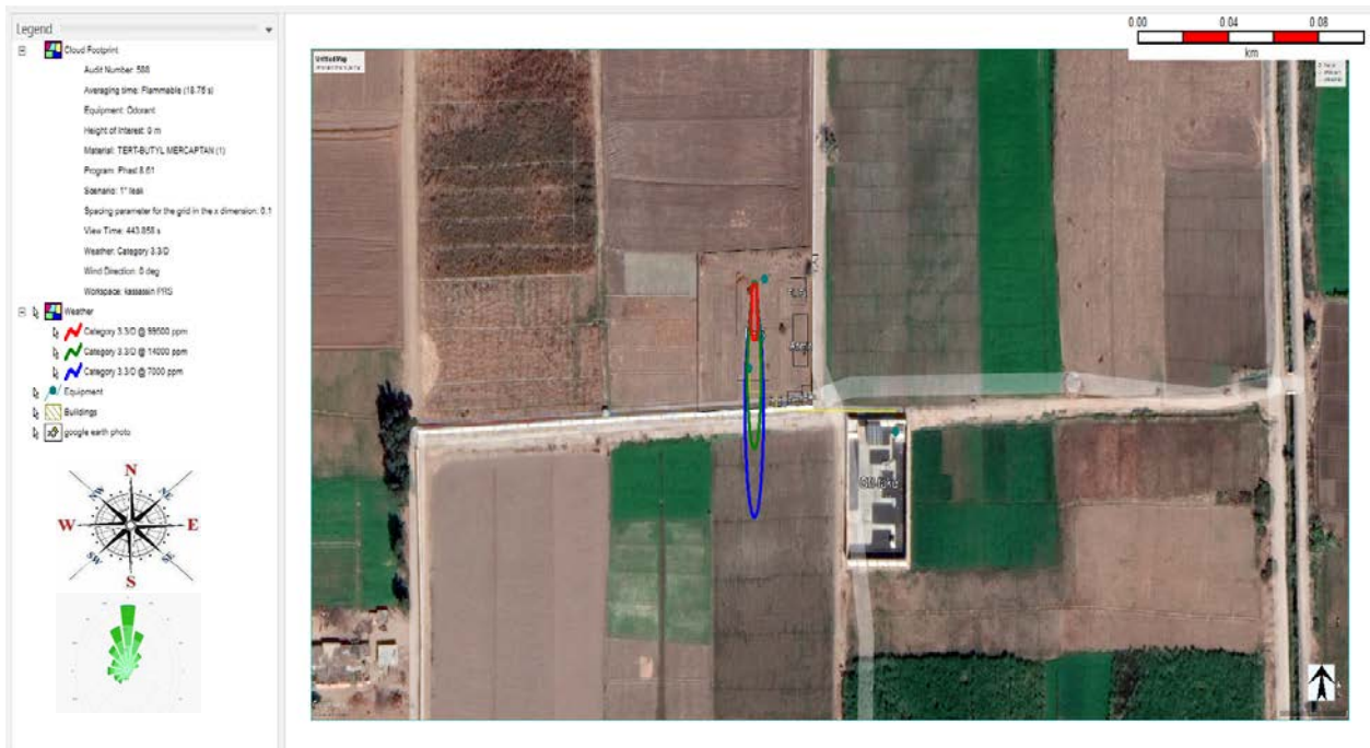
Figure 31. Cloud Footprint (UFL/LFL) on site (Odorant leak)
