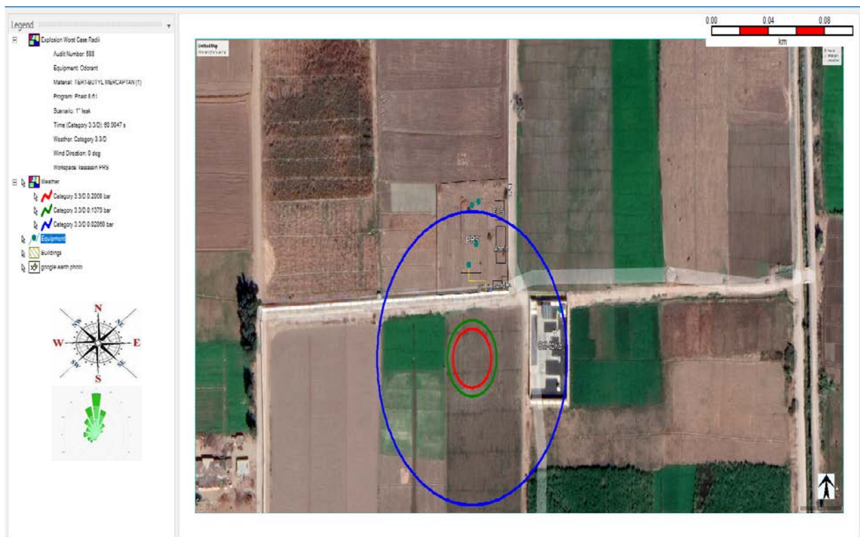
Figure 35. Explosion Overpressure Waves on Site (Odorant Leak)
