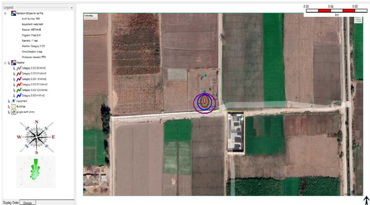
Figure 38. Heat Radiation Contours - Fire on Site (Gas Heater)
