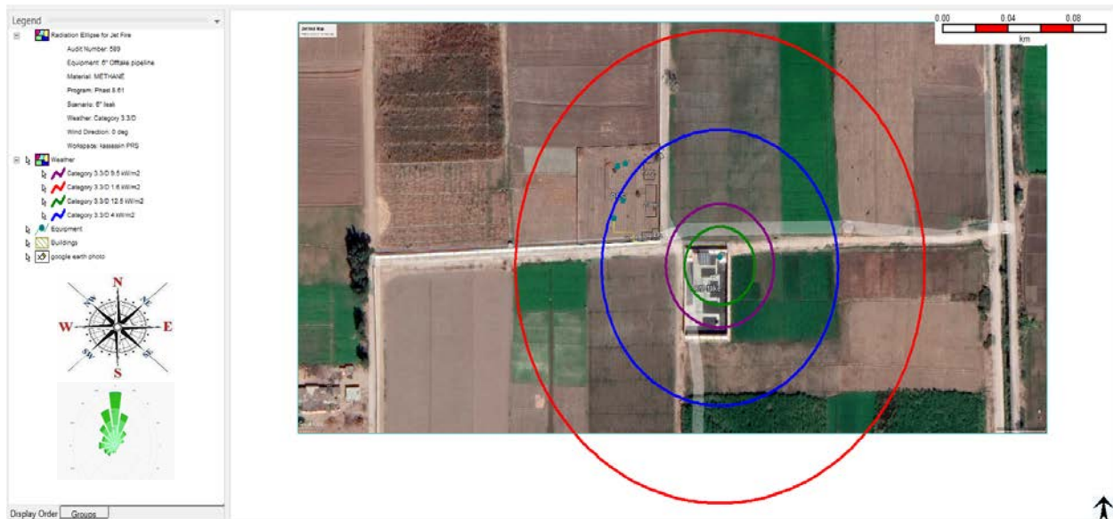
Figure 46. Heat Radiation Contours from Jet Fire (6" off-take Pipeline Full Rupture)
