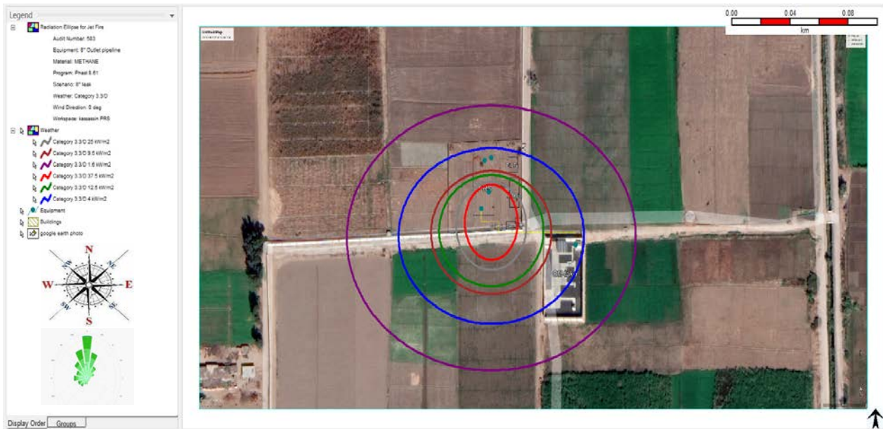
Figure 27. Heat Radiation Contours from Jet Fire (8'' Outlet Pipeline Full Rupture)
