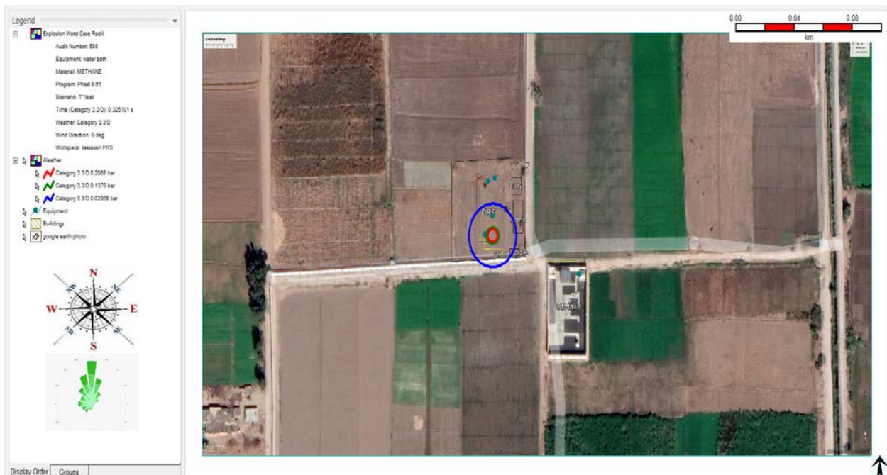
Figure 40. Explosion Overpressure Waves on Site (Gas Heater)
