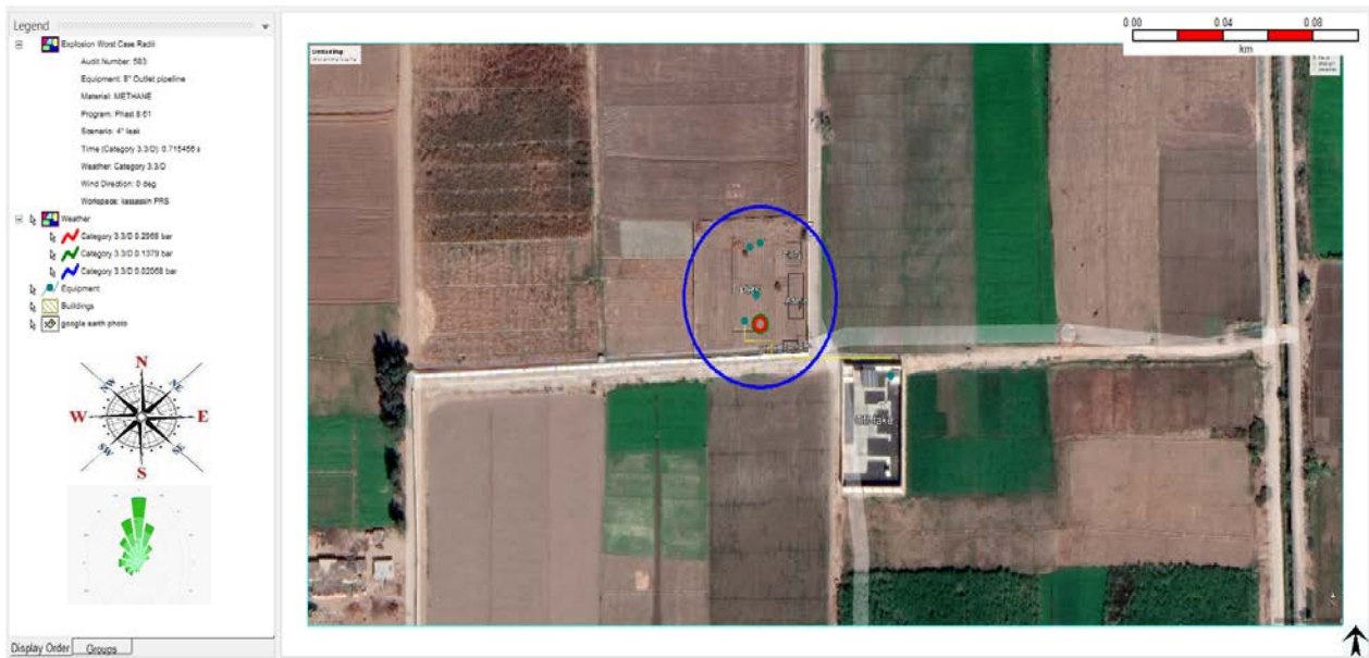
Figure 25. Worst-Case Explosion Overpressure Waves (4'' hole in 8'' Outlet Pipeline)
