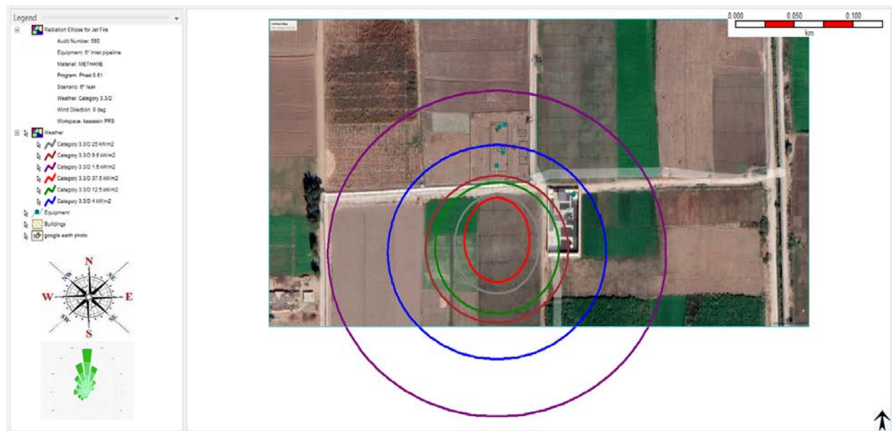
Figure 19. Heat Radiation Contours from Jet Fire (6'' Inlet Pipeline Full Rupture
