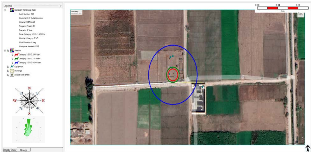
Figure 28. Worst-Case Explosion Overpressure Waves (8" Outlet Pipeline Full Rupture)
