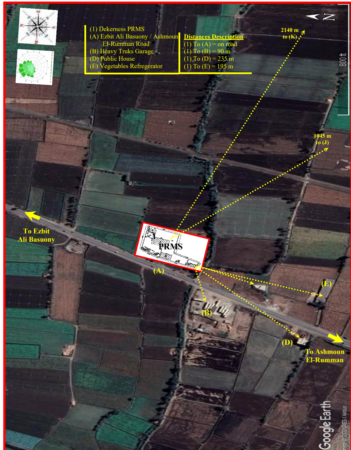
Figure (13) Dekerness PRMS / Offtake Distances to the Nearest Surroundings Plotted on Google Earth Photo
