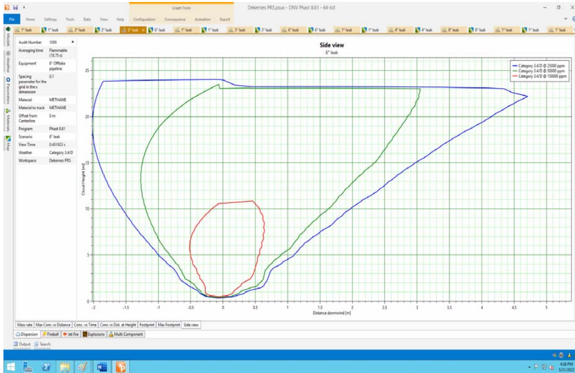
Figure (42) Gas Cloud Side View (UFL/LFL) (6" off-take Pipeline Full Rupture)
