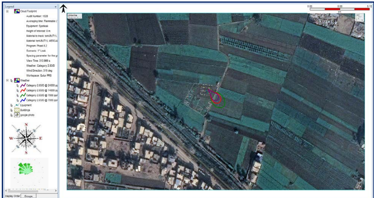
Figure 31. Cloud Footprint (UFL/LFL) on site (Odorant leak)
