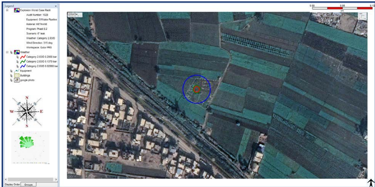
Figure 47 Explosion Overpressure Waves (6" off-take Pipeline Full Rupture)
