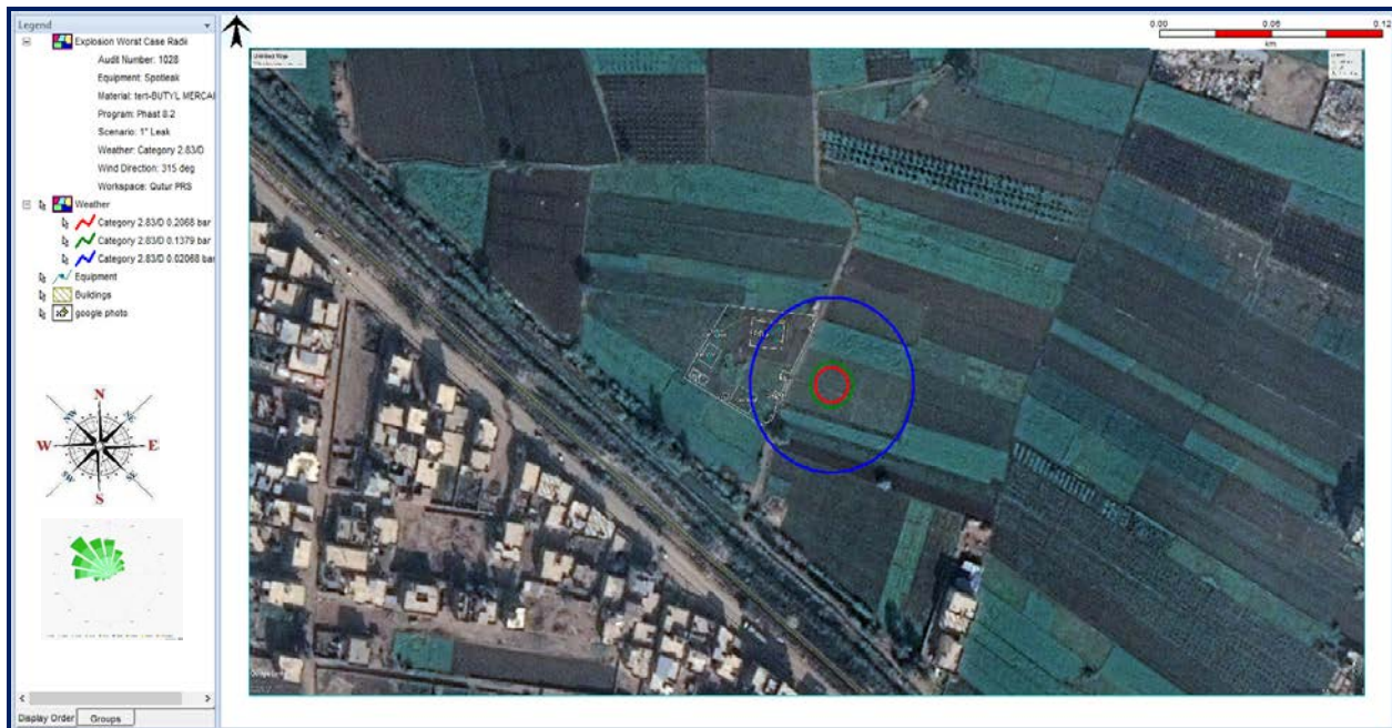
Figure 35. Explosion Overpressure Waves on Site (Odorant Leak)
