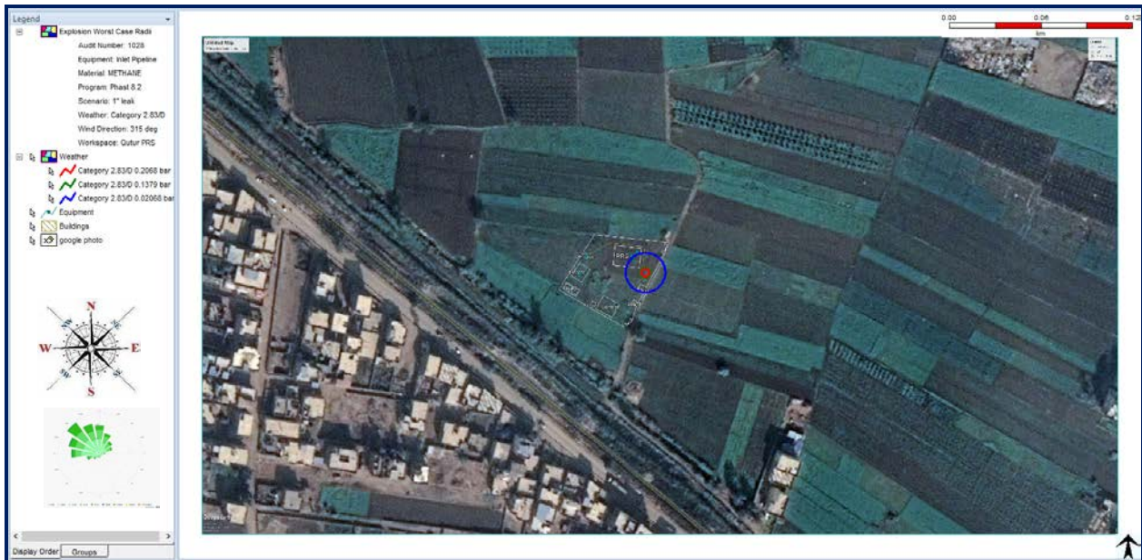
Figure 15 Explosion Overpressure Waves (1" hole in 4" Inlet Pipeline)
