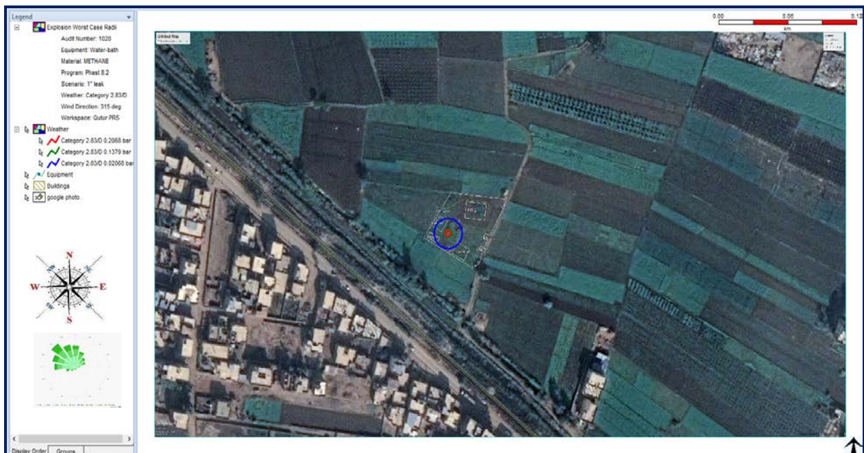
Figure 40. Explosion Overpressure Waves on Site (Gas Heater)
