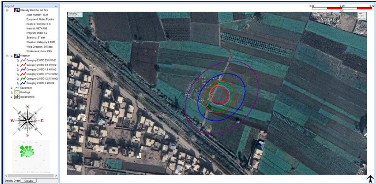
Figure 27. Heat Radiation Contours from Jet Fire (6'' Outlet Pipeline Full Rupture)
