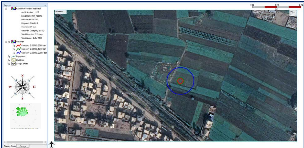
Figure 18. Explosion Overpressure Waves (2" hole in 4" Inlet Pipeline)
