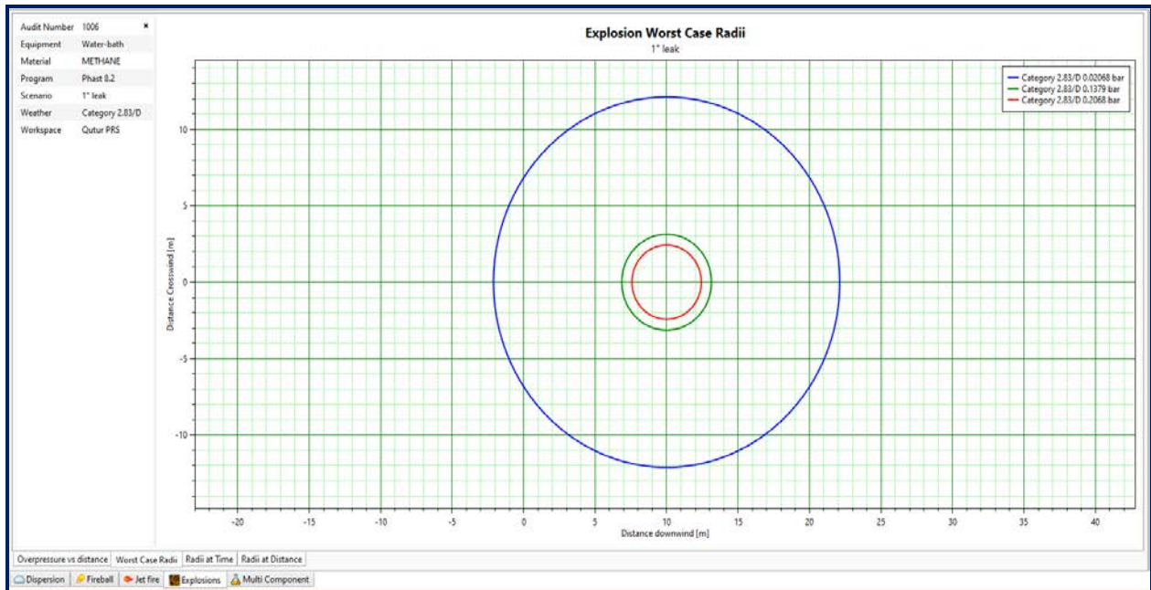
Figure 39. Explosion Overpressure Waves Graph (Gas Heater)
