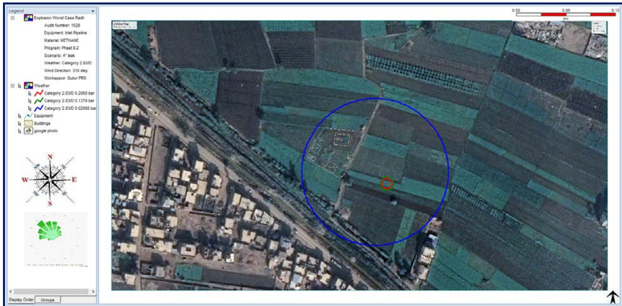
Figure 21. Explosion Overpressure Waves (4" Inlet Pipeline Full Rupture)
