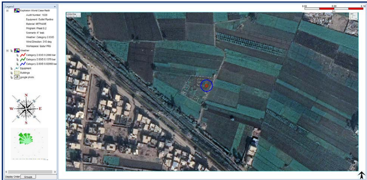
Figure 28. Explosion Overpressure Waves (6" Outlet Pipeline Full Rupture)
