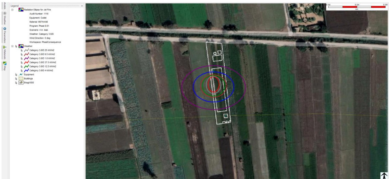
Figure 22. Heat Radiation Contours from Jet Fire (4" hole in 10" Outlet Pipeline)
