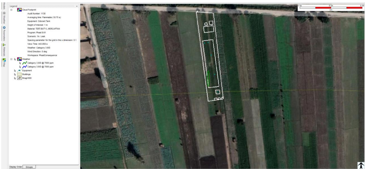
Figure 29. Cloud Footprint (UFL/LFL) on site (Odorant leak)
