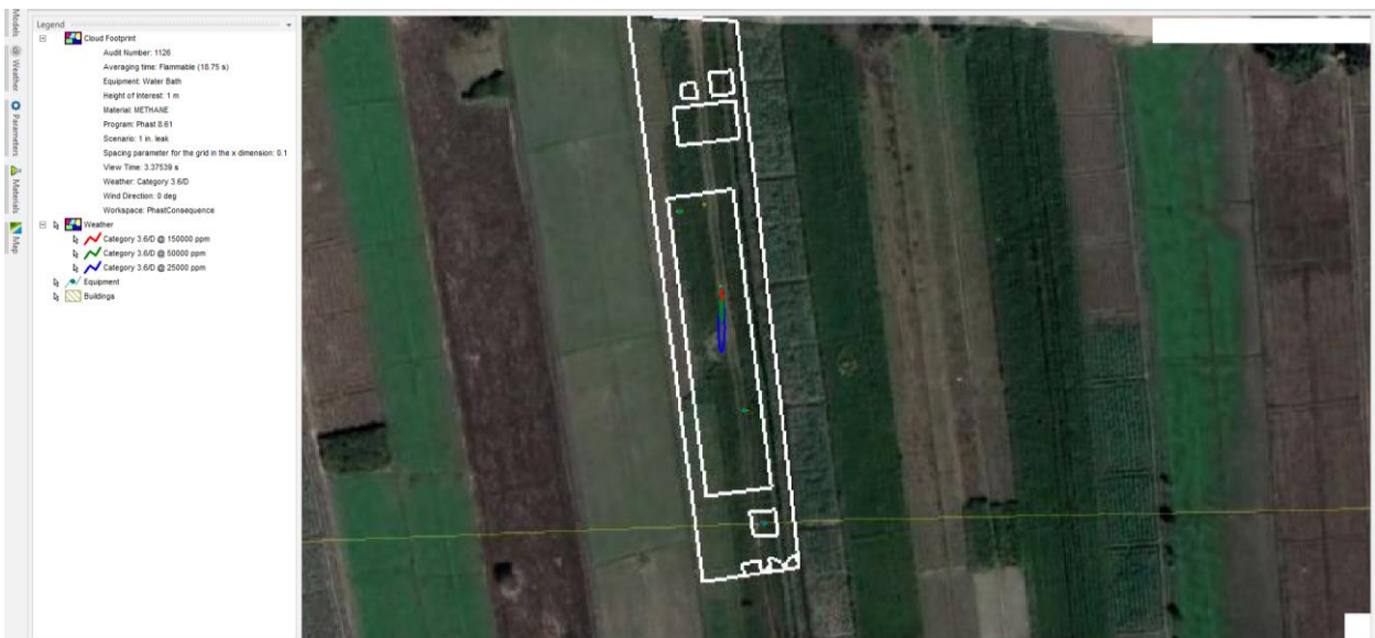
Figure 35. Cloud Footprint (UFL/LFL) on site (Gas Heater)
