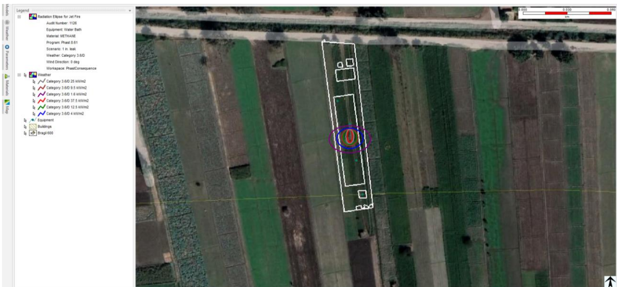
Figure 37. Heat Radiation Contours - Fire on Site (Gas Heater)
