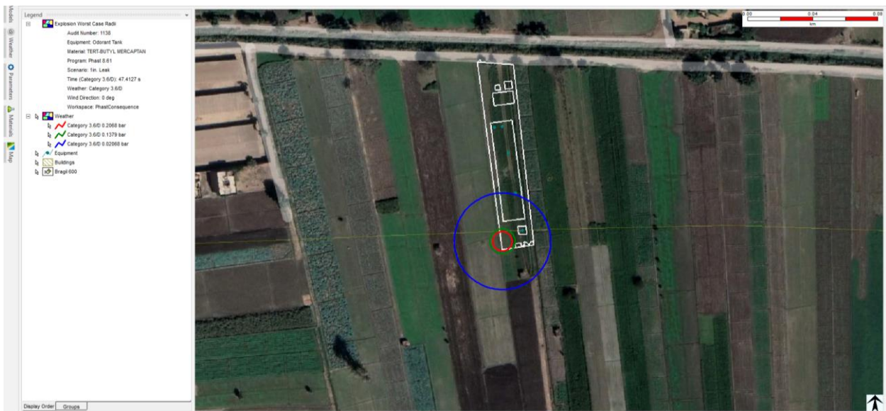
Figure 33. Worst-Case Explosion Overpressure Waves on Site (Odorant Leak)
