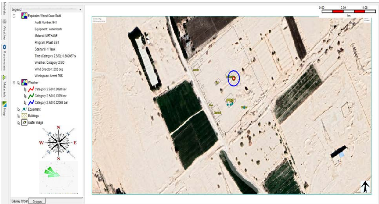
Figure 41. Explosion Overpressure Waves on Site (Gas Heater)
