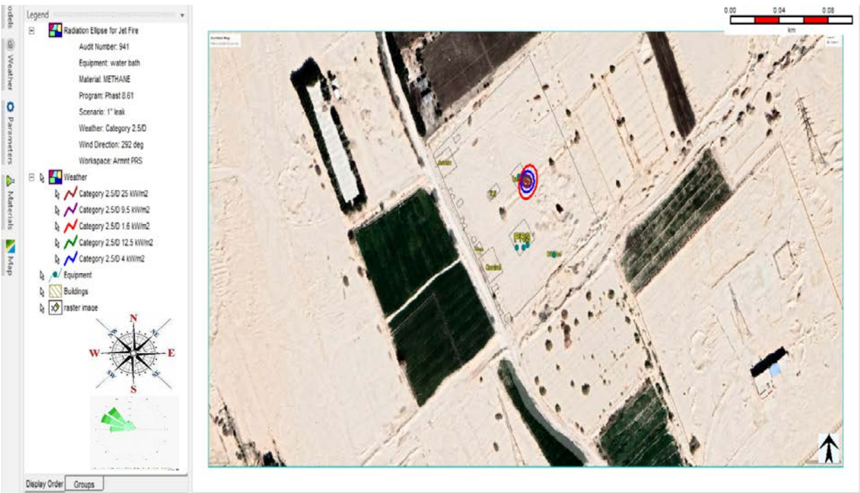
Figure 39. Heat Radiation Contours - Fire on Site (Gas Heater)
