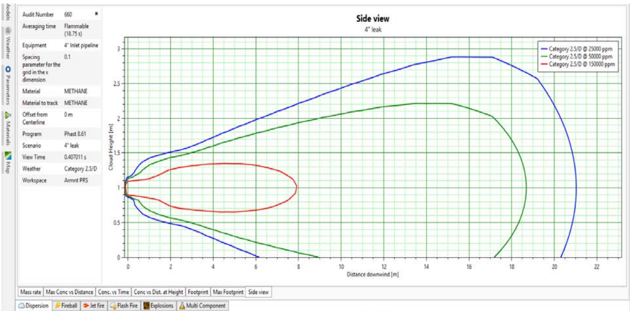
Figure 19. Gas Cloud Side View (UFL/LFL) (4" Inlet Pipeline Full Rupture)
