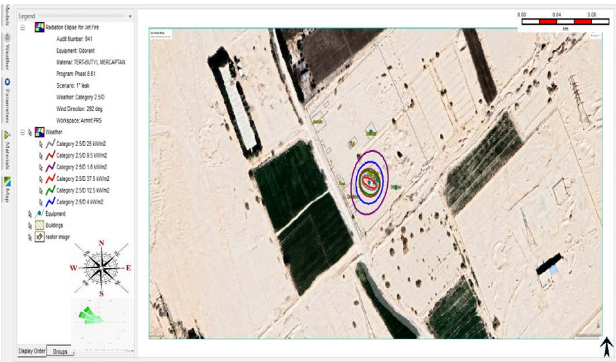
Figure 34. Heat Radiation Contours - Jet Fire on Site (Odorant Leak)
