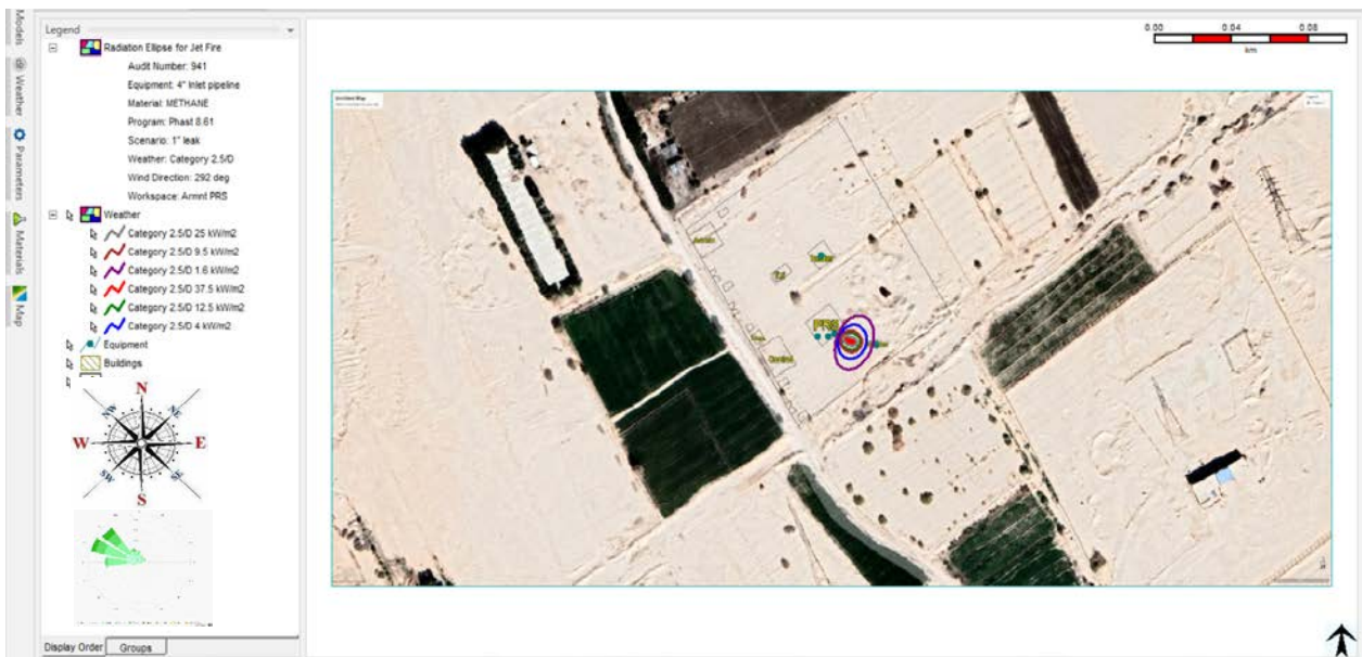
Figure 14. Heat Radiation Contours from Jet Fire (1" hole in 4" Inlet Pipeline)
