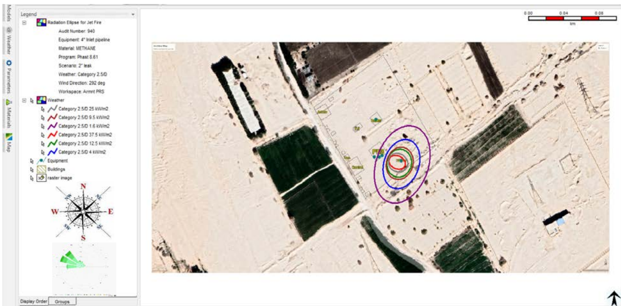
Figure 17. Heat Radiation Contours from Jet Fire (2" hole in 4" Inlet Pipeline)
