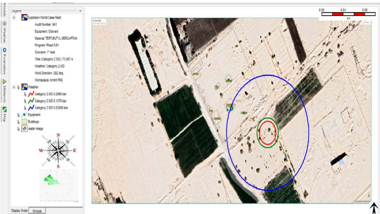
Figure 36. Explosion Overpressure Waves on Site (Odorant Leak)
